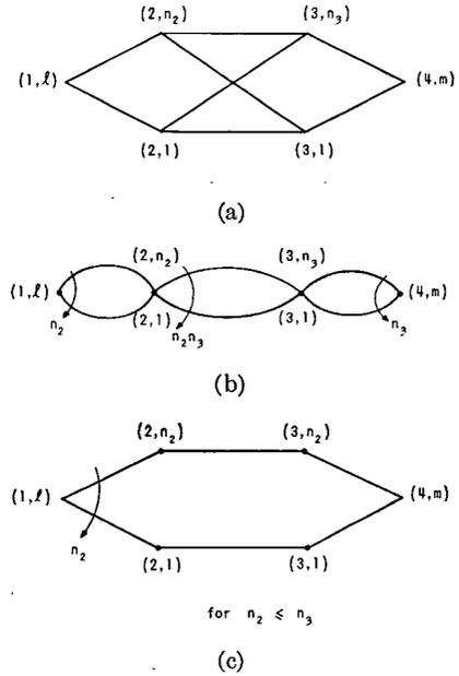
Fig. 7. (a) 4-stage network. (b) Graph for  $B_0$ . (c) Graph for  $B_1$ .
